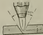
FIG. 3. Position of the torch, the point of the flame penetrating into the angle formed by the sheets
